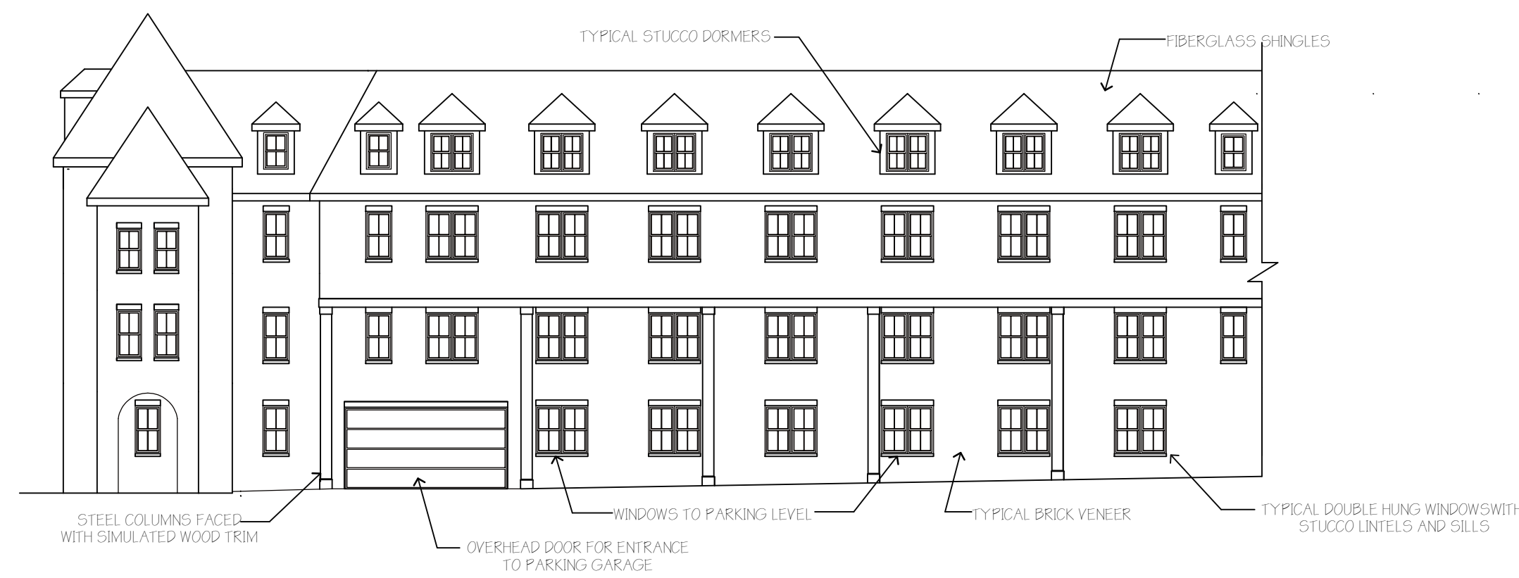
MAIN COURTYARD LEFT SIDE ELEVATION
