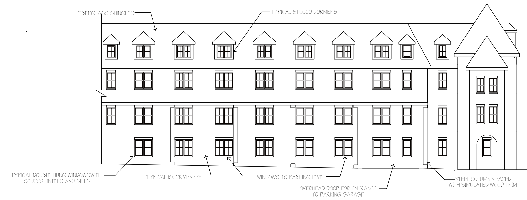
MAIN COURTYARD RIGHT SIDE ELEVATION
